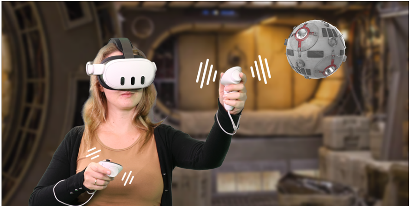
Figure 1: A user wearing a VR head-mounted display utilizes handheld controllers with adaptive vibrotactile feedback to detect and locate a remote object in 3D space. The intensity of vibrations in each controller varies based on the object's relative position, mimicking auditory localization mechanisms to enhance spatial awareness.
